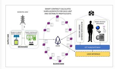
The relationships between the power grid, blockchainbased smart contracts which automatically rank and distribute incentives to each unit, and the end user interface within the home.
