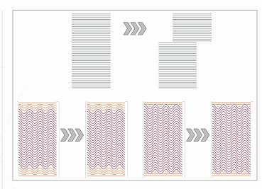
Traditional FDM 3D printing produces products subject to damage by shearing due to weaknesses between the layers of the print (top). By using corrugated layers (indicated in maroon) 3D printed products can avoid damage by shearing (bottom). Transitional layers (indicated in orange) ensure that the top and bottom of corrugated prints are just as smooth as would be expected from any other FDM print.
