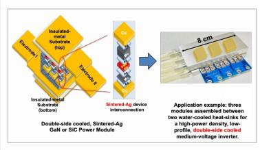
Illustration of the new, innovative packaging concept involving interconnection on both sides of the device achieved by our patented silver-sintering material for double-sided cooling which enables more than 50% more effective heat extraction and significantly lower electrical parasitics.
