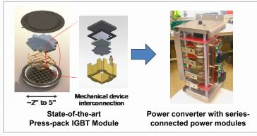
Example of a state-of-the-art packaging of a medium-voltage power module of silicon-based device where the interconnection to the device chips is achieved by mechanical press-contact resulting in high electrical and thermal resistance.
