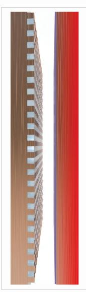
Diagram of the planar bridging-droplet thermal diode. The vapor chamber is comprised of a wick structure (red plate on the left) and an opposing plate (brown on the right) with a smooth hydrophobic coating (blue film). The box on the left shows the forward mode in which dropwise condensate bridges across the gap to return to the wicked evaporator. On the right is a schematic of the reverse mode in which the hydrophobic side is heated and the liquid is trapped in the opposing wick.
