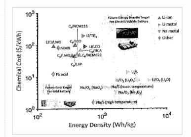
Plot of chemical cost vs. energy density for potential chemical battery options.
