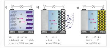
Illustrated operating principles of lithium-ion (left), metal-oxygen (middle), and metal-sulfur (right) battery discharge (Beilstein Journal of Nanotechnology).
