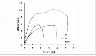
Compatibilization of 50:50 blends increases modulus from 820 MPa to 1200 Mpa and strain at break from 2% to 5%.
