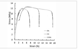
Compatibilization of 80:20 blends increases strain at break from 7% to 19% without affecting modulus.
