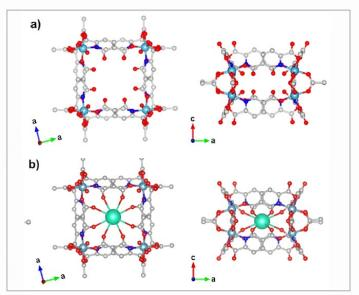
Crystal structure of the molecular cage obtained from Single-Crystal X-Ray Diffraction (SCXRD) with (a) and without (b) a complexed Cs+ ion.
