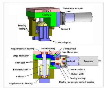
A detailed design of the energy harvester inside the invented energy harvesting tie.
