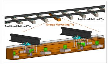
The overall design of the invented energy harvesting railroad tie. It has similar dimensions to a conventional railroad tie so it can be installed and maintained in the same manner as a standard tie on the track.
